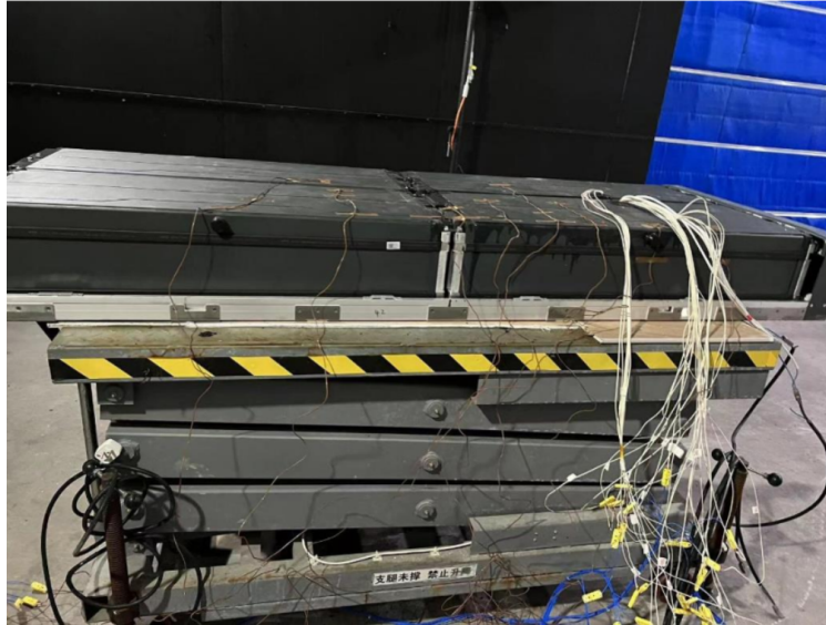
Figure 8: A module prepared for the UL 9540A test. This image was taken from the UL 9540A module-level test report [4].
