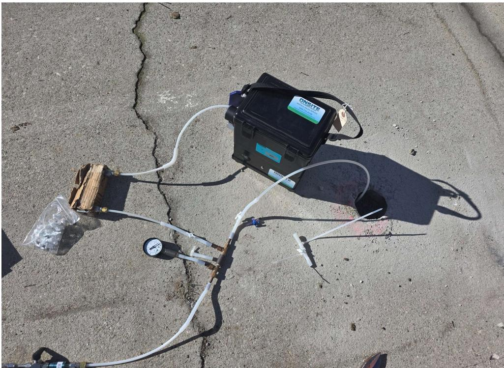
**Photo 6** View of soil gas sampling train.
