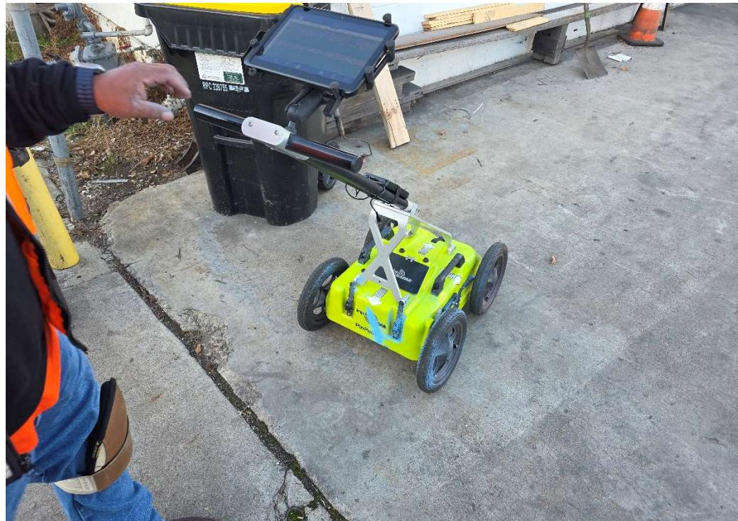
**Photo 2** View of ground penetrating radar used during the geophysical survey.
