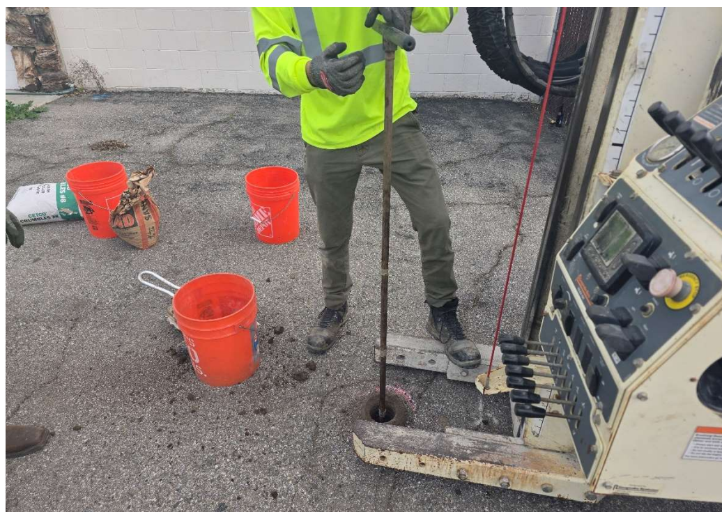
Photo 2 View of hand augering at SGP-1.
